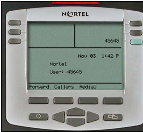
Figure 10: Logged on to an IP Audio Conference Phone 2033 using an IP Phone 2004
